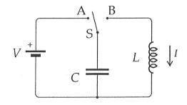
A3 Switch S has been in position A for a long time, causing the capacitor to be completely charged. At t=0, the switch is thrown to position B, and we measure the maximum current  $I_{\rm max}$ . Give an expression for L in terms of the quantities V, C, and  $I_{\rm max}$ .
