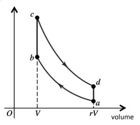
$$\begin{aligned} \underline{ANSWER} \\ Q^{a \to b} &= 0 \\ Q^{c \to d} &= 0 \end{aligned} \qquad Q^{b \to c} = nC_V(T_c - T_b) > 0 \\ Q^{c \to d} &= 0 \end{aligned} \qquad Q^{d \to a} = nC_V(T_a - T_d) < 0 \end{aligned}$$
