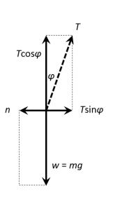
$n = T \sin \varphi \quad \text{and} \quad mg = T \cos \varphi$  $\sin \varphi = \frac{16}{30 + 16} \quad \Rightarrow \quad \varphi = 20.354^{\circ}$  $\frac{n}{mg} = \tan \varphi \quad \Rightarrow \quad n = mg \tan \varphi = 164 \text{ N}$  $T = \frac{mg}{\cos \varphi} = 470 \text{ N}$
