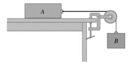
Two block are connected by a massless cord which rolls over a massless and frictionless pulley. Block A sits on a level, frictionless surface, and is sliding to the right. The masses of the blocks A and B are  $m_A = 7$  kg and
