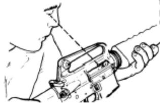
5. With the selector lever pointing toward SAFE allow the bolt to go forward by pressing the upper portion of the bolt catch.
