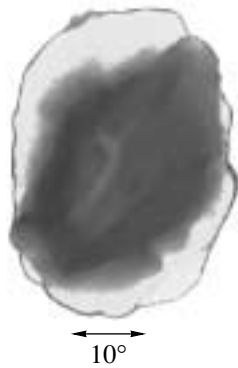
Fig. 9. Typical image of a proton beam observed traveling in the forward direction from the interaction of a high-intensity laser with a 1.8- \mu\text{m} -thick aluminum foil. The proton beam passed through a 25- \mu\text{m} Mylar filter, corresponding to an energy above 1.2 MeV. The laser intensity on the target is 2 \times 10^{18} \text{ W/cm}^2 at 2\omega_0 illumination normal to the target.
