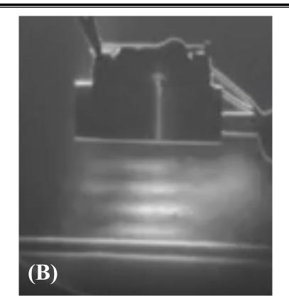
*Figure 2*: Using schlieren imaging we can see sound waves, which are varying pressure waves. This is done by having the flashlight strobe at the same frequency of the sound wave, allowing the camera to always see the same spatial pattern. (A) traveling sound wave; (B) standing sound wave. Reference: Harvard Natural Sciences Lecture Demonstrations Schlieren Optics.
