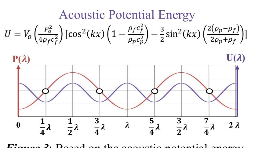
*Figure 3*: Based on the acoustic potential energy, we can predict that the Styrofoam balls tend to move toward the nodes (o) of the pressure wave.
