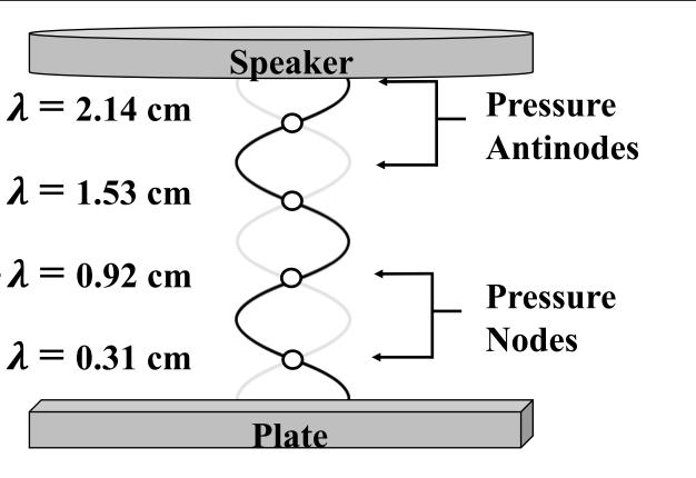
Figure 4: A geometric representation shows the expected vertical positions relative to the plate. Reference: Acoustic Levitation and the Acoustic Radiation
