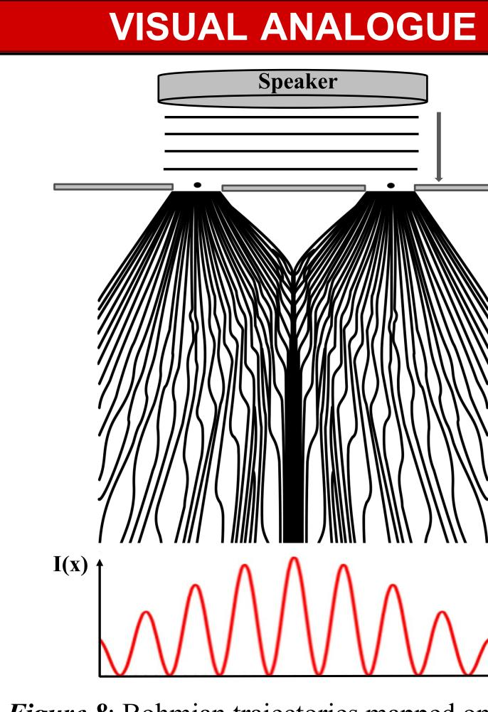
*Figure 8*: Bohmian trajectories mapped onto an acoustic double-slit system with Styrofoam balls. Below is the corresponding intensity pattern that is formed by the particles following the trajectories.
