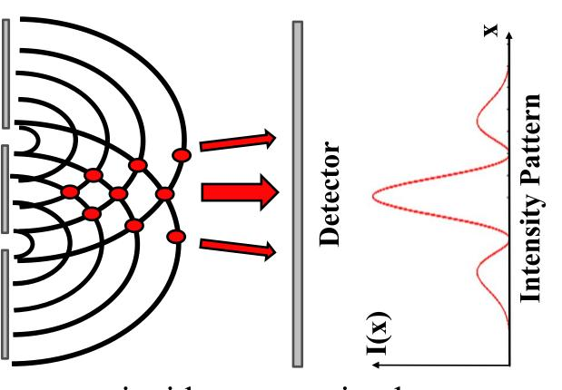
*Figure 6*: Shows an incident acoustic plane wave diffracting as it passes through a double-slit. Interference of the acoustic waves causes an intensity pattern that is shown on the right side.
