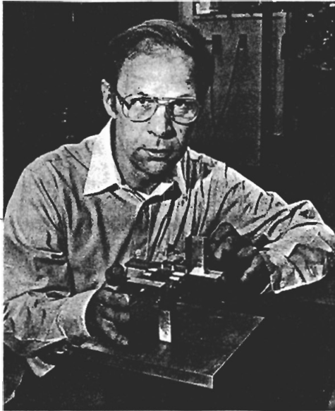
Duane Jaecks with knife-edge apparatus he will use to measure focal length variations in telescopes.
